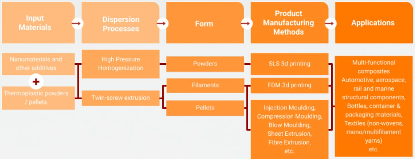
Process flow for the manufacture of Versarien’s Polygrene™-Thermoplastic compounds/masterbatches and their downstream products
