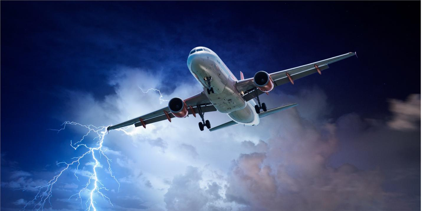
Lightning strike is an extreme high-energy impulse lasting 1-10 $\mu$ sec which induces an electrical pulse of 1 billion volts and current of 10k-200kA, and a thermal spike of up to 30,000 $^{\circ}$ K. Due to the short time duration, the overall power is minimal, and overall temperature rise of up to 50 $^{\circ}$ C. However, the strike can cause extreme mechanical damage and even loss of an aircraft due to structural damage to flight surfaces.
