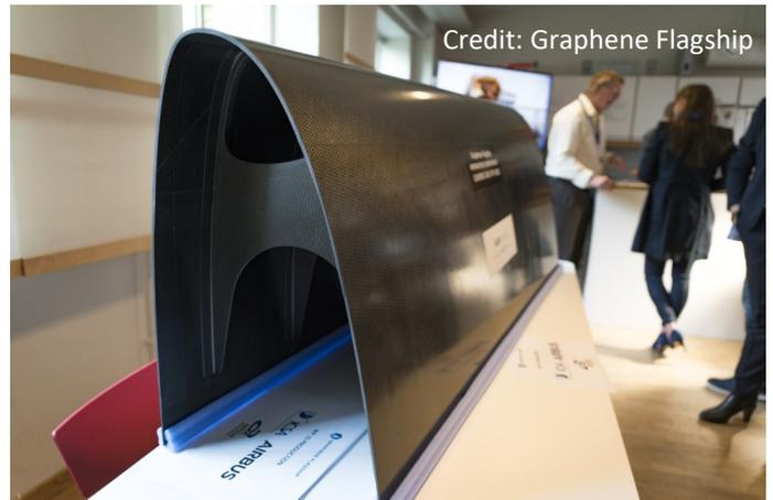
reduction. Specifically, the presence of a small amount of graphene can significantly reinforce both thermoplastic and thermosetting systems through stress transfer at the filler-matrix interfaces, which allows the components to bear more load [2-3]. Over the past decade, graphene has been hybridised into CFRP composites and shown to facilitate the interfacial bonding between the fibre and resin system and result in further mechanical reinforcement.
